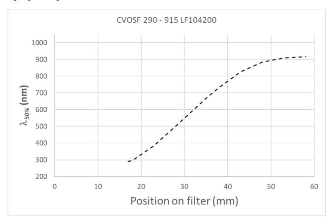
NOTE: If the filter is being used for wavelengths above ~900 nm it is important to ensure that the 1<sup>st</sup> order wavelength is at least ~5% longer than the filter edge wavelength for the upper part of the wavelength range.
