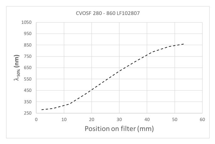
NOTE: If the filter is being use for wavelengths above ~1000 nm it is important to ensure that the 1<sup>st</sup> order wavelength is at least ~22% longer than the filter edge wavelength for the upper part of the wavelength range.
