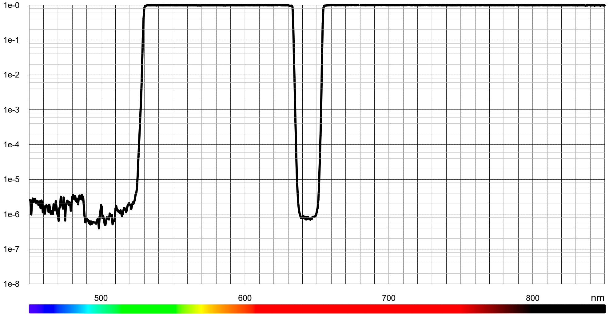
Typical transmission LP530 N642 (LF104708)
