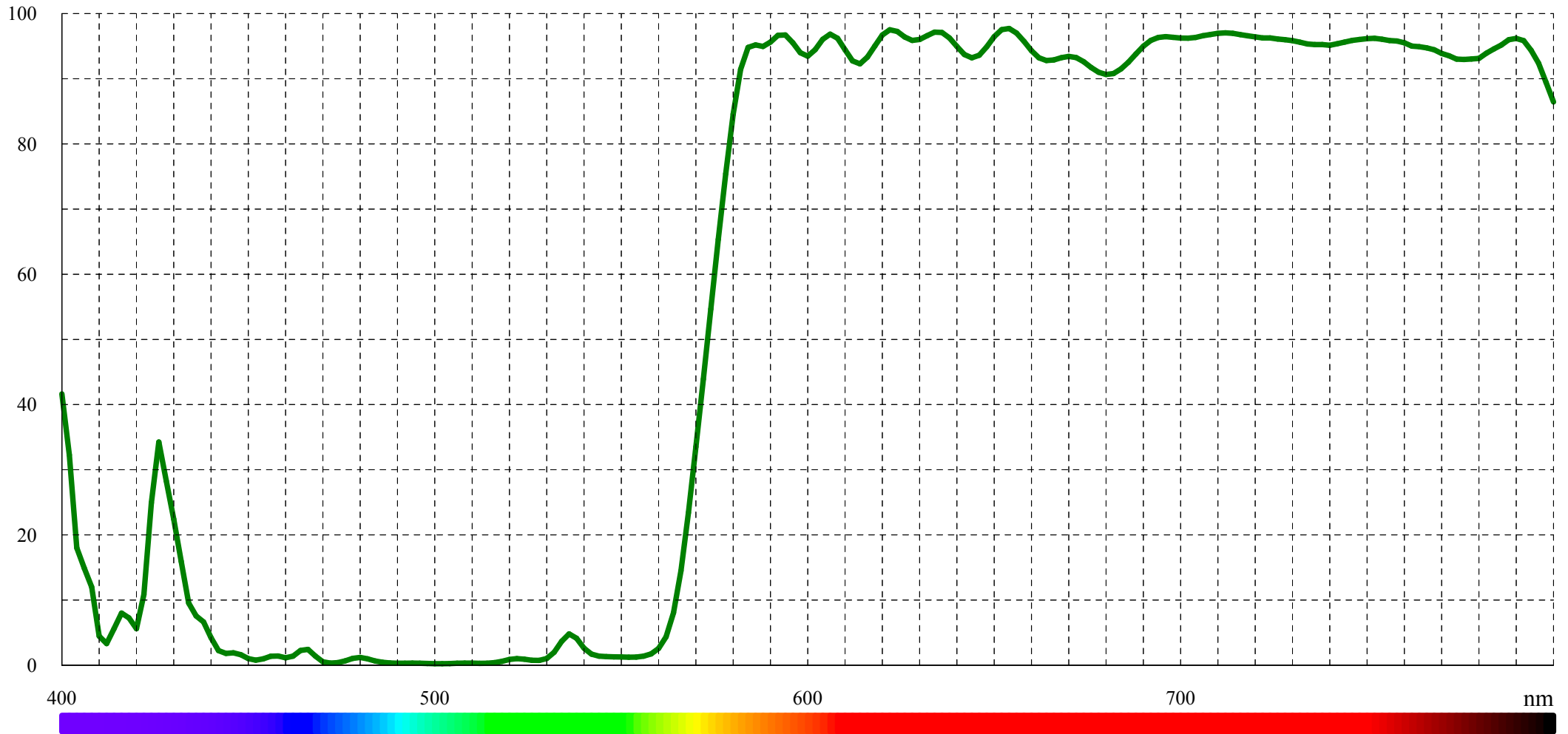
Typical transmission for DCLP 580 (LF101593)
